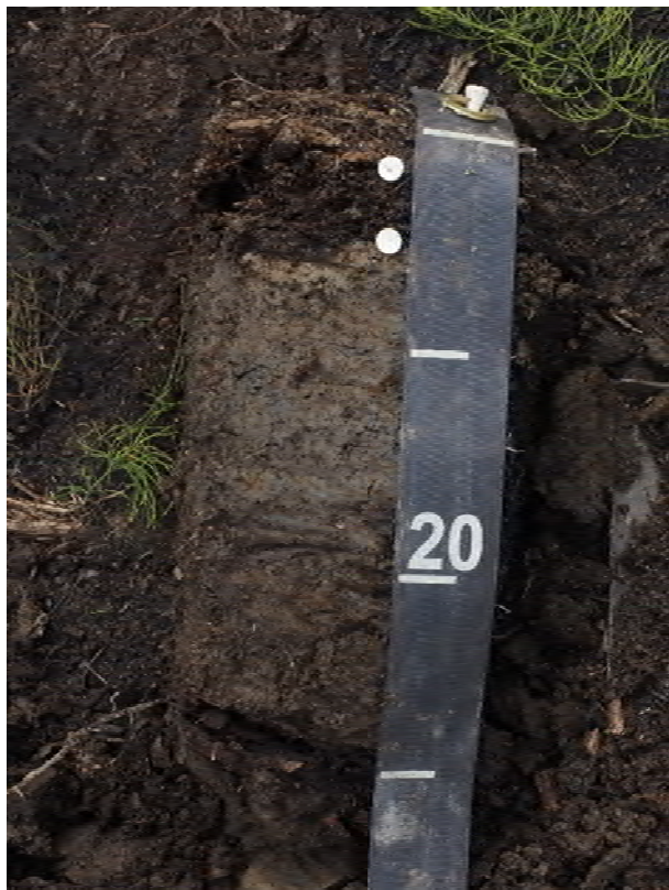
Figure 27. Soil profile at the Isom Creek fire, dark surface horizon is mostly charcoal and wood ash,
