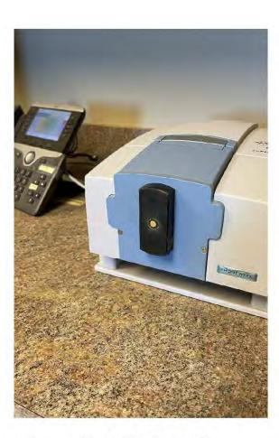
Figure 1 - A Bruker Alpha-II MIR spectrometer scanning a sample. The surface area is the same as the end of a pencil eraser; four subsamples are scanned per horizon.
